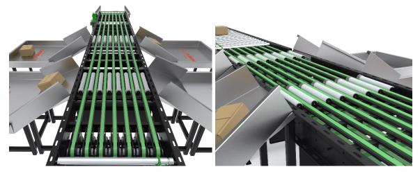
Our Narrow Belt Sorter was designed for smooth 90° transfer of small sized materials. A series of long narrow belt are used to transfer material while the roller system delivers the required shipments to the allocated stations.
